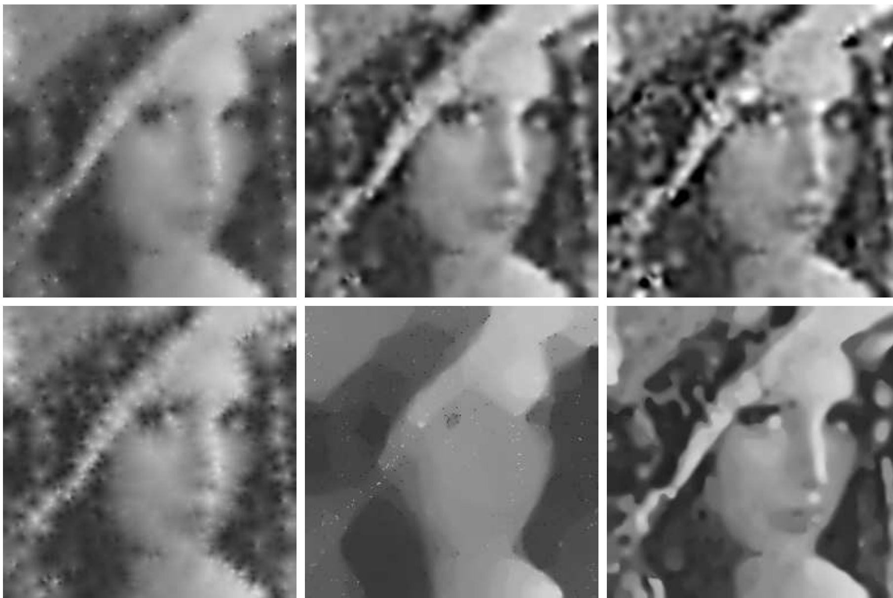
Impact of the PDE on the interpolation result. (a) Top left: Interpolation by linear diffusion. (b) Top middle: Biharmonic smoothing. (c) Top right: Triharmonic smoothing. (d) Bottom left: AMLE. (e) Bottom middle: Isotropic nonlinear diffusion. (f) Bottom right: EED.
