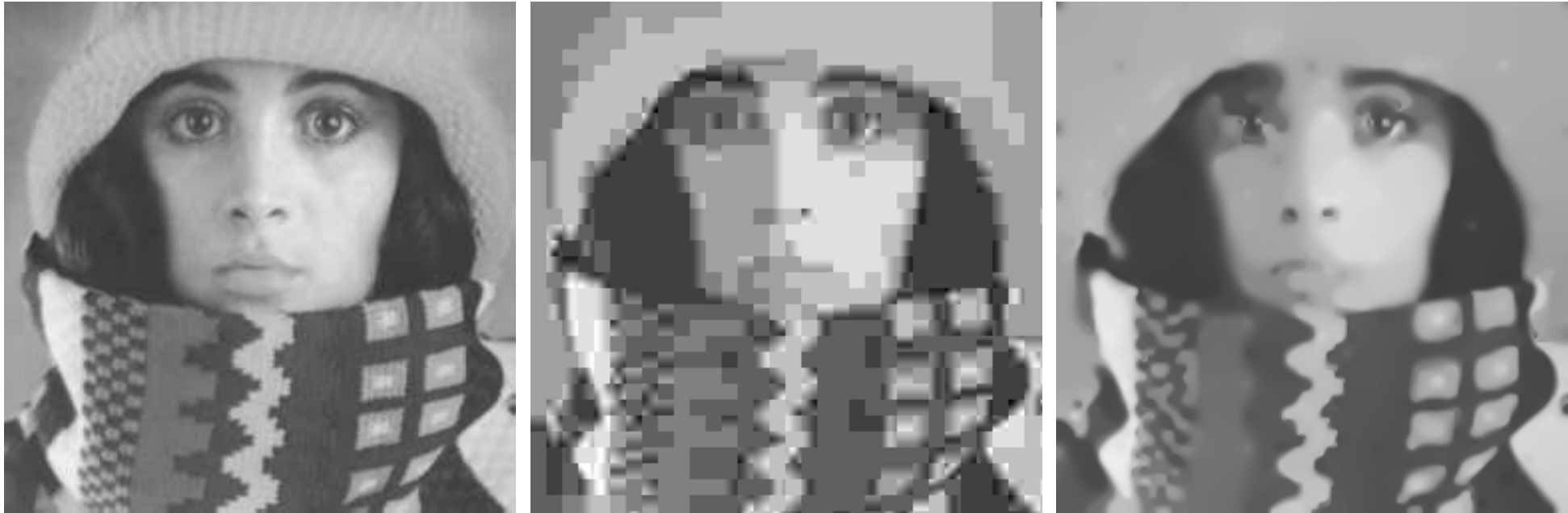
Comparison at high compression rate (40:1). (a) Left: Original image. (b) Middle: JPEG. (c) Right: EED-based compression.
